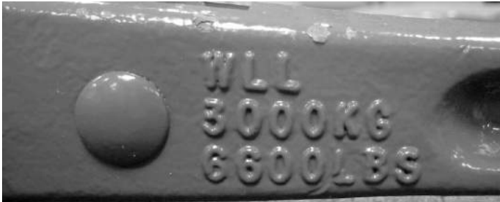
Indicator of Working Load Limit
