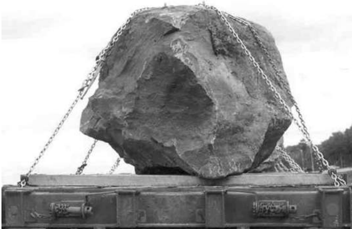
Chain is used to secure large boulders
